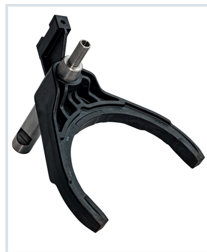
Fig. 1. An operating temperature of 120°C creates harsh conditions. The maximum permissible deformation of the fork-ends under an acting force of 1500N was well below 0.8mm (© GK Concept)
